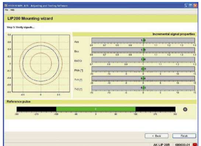
Commissioning using PWM 20 and ATS software
