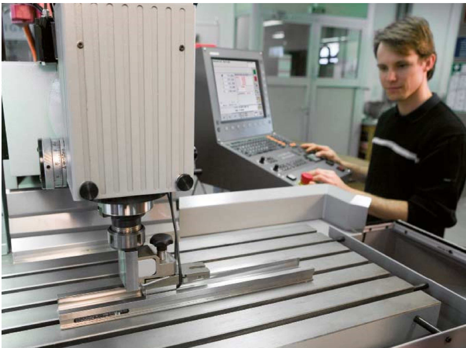
Determining the positioning accuracy with a VM 182
