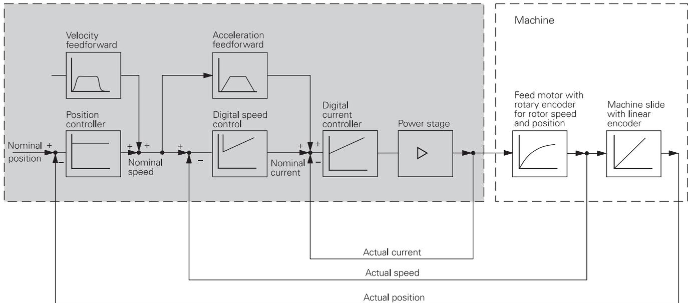
**Axis feedback control** The TNC 640 can be operated with following error or feedforward control. During roughing operations at high speeds, for example, you can switch to velocity semi-feedforward control via an OEM cycle in order to machine faster at reduced accuracy.
