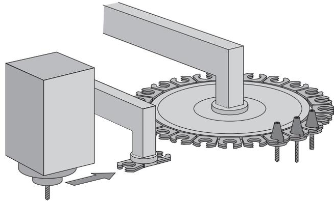
**PLC axes** Axes can be defined as PLC axes. They are programmed by means of M functions or OEM cycles. The PLC axes are positioned independently of the NC axes.
