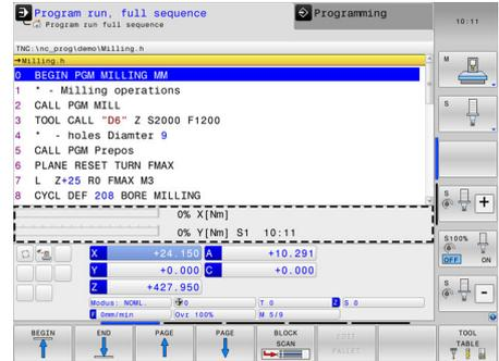
**PLC soft keys** The machine manufacturer can display his own PLC soft keys in the vertical soft-key row on the screen.
